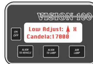
**THE EXAMPLE (LEFT) SHOWS THAT THE LAMP DOES REQUIRE VERTICAL ADJUSTMENT TO BE WITHIN STATE SPECIFICATIONS.**
