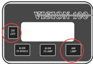
**STEP 1:** With the aimer ON and with the front cover down and with the headlamps ON and at low beam, press the "AIM LAMP" button.
